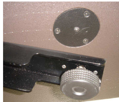
(6) Rotate the pivoting arm into position
