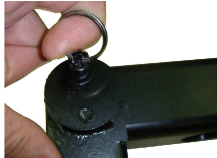
(2) Release pivoting arm locking pin
