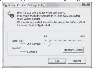
A sufficiently large buffer size decreases the chance of sound dropout (sound interruption) but increases audio signal transmission delay (latency).
