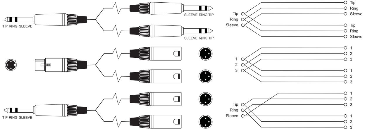
**Headphone Separator** Note: for every doubling of headphones the load impedance is halved. Do not go below 150 Ohms.
